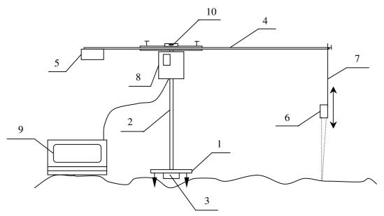
Fig. 1. Schematic diagram of profilograph design
